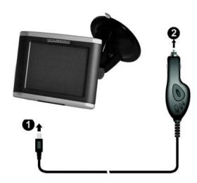
To connect the charger, insert the terminal (1) into the connector on the navigator and terminal (2) into the car's cigar lighter socket.
